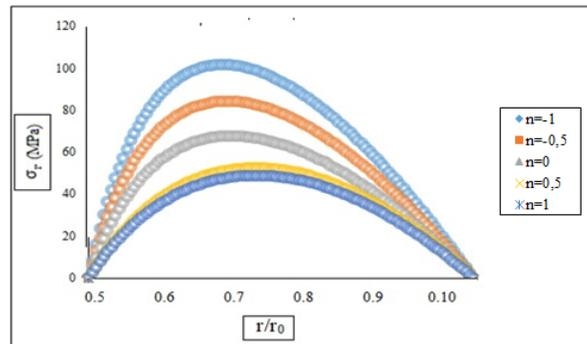
**Figure 3.** Radial stresses occurring in an angular (50 rad/sec) rapidly rotating Silicon karbür (SiC) material cylinder.
