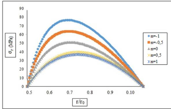
**Figure 2.** Radial stresses occurring in an angular (50 rad/sec) rapidly rotating Bor karbür (B4C) material cylinder.
